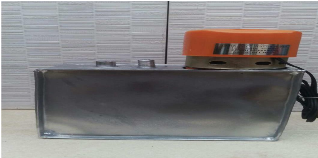
Figure (3) External Tank and Water Pump
